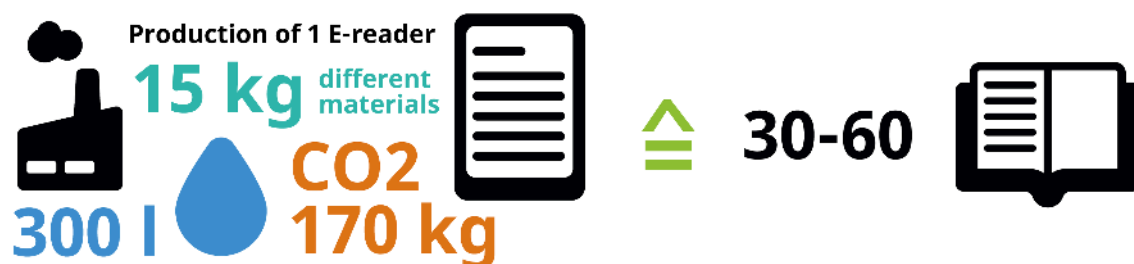
Figure 4: To produce one e-reader, 15 kilograms of different materials, 300 liters of water, and 170 kilograms of the greenhouse gas carbon dioxide are needed. If you read fewer than 30–60 books on the e-reader device, it may be environmentally better to read the paper books. (Image from KDE published under a CC-BY-SA-4.0 license. Design by Lana Lutz.)
